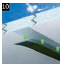
10 Posa in opera delle lamine in CFRP Sika® CarboDur®.
